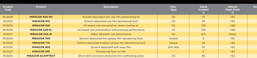
600 number is oil film 700 number is grease film 800 number is wax film
